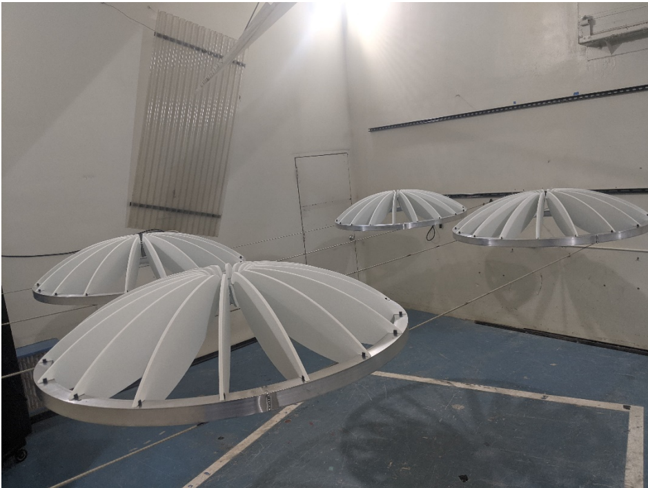
Figure 4 – Specimen mounted in test chamber, staggered spacing between rows
