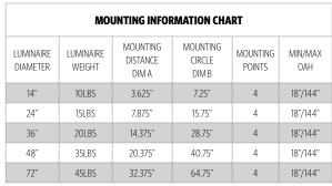
$^{\star}$  PIEM & PIEC ships with one of three standard OAH's (48", 100" or 144") field adjustable to the desired height.
